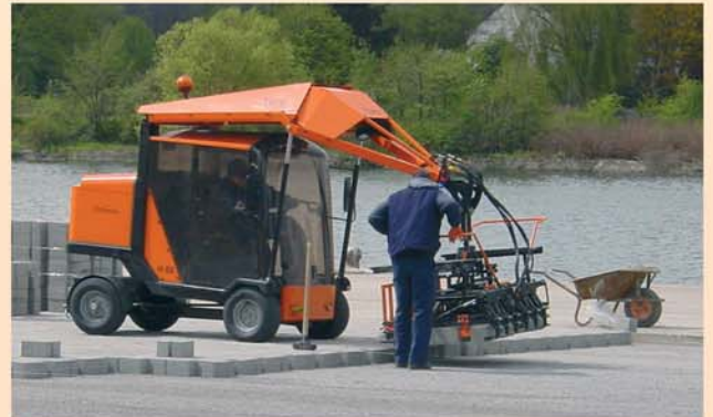
Heavy duty chassis and boom for longterm durability in extrem working conditions ( photo: paver layer 1,2 m 2 , height 13cm - weight approx. 350 kg).
