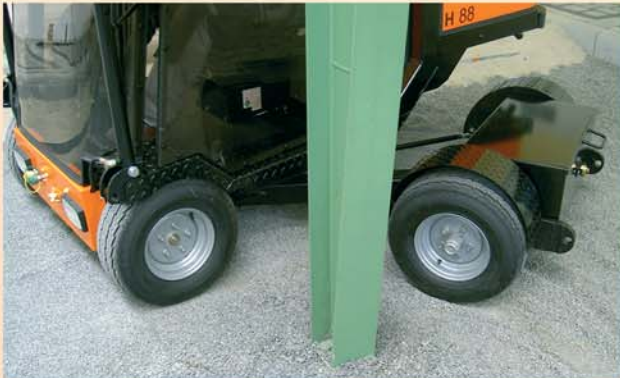
Extreme maneuverability provided by an inner radius of just 800 mm and excellent stability.
